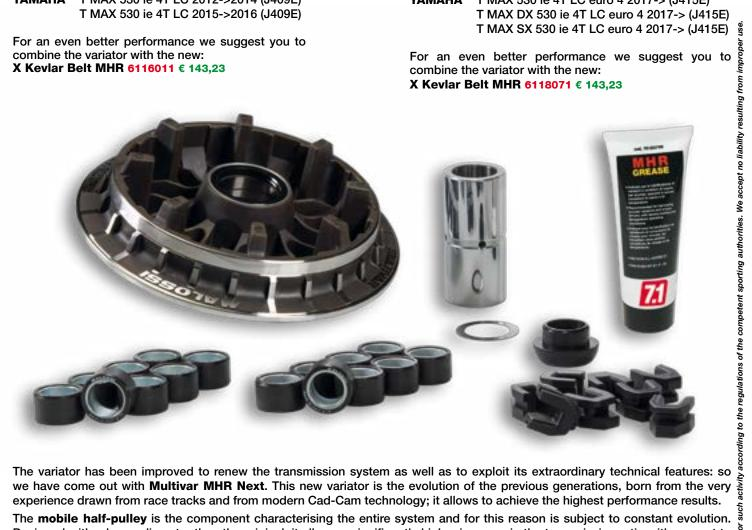
The **mobile half-pulley** is the component characterising the entire system and for this reason is subject to constant evolution. Designed with a larger diameter than the original, it allows a significantly higher increase in the transmission ratio with respect to the original pulley.
